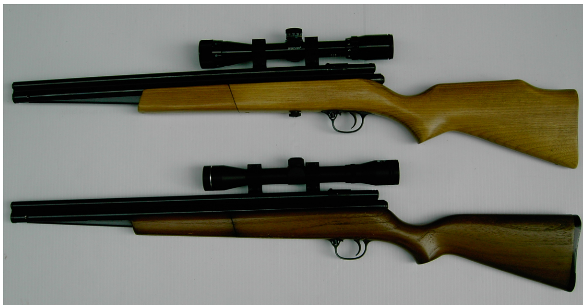
Top rifle is a Sears J.C. Higgins variant of the Crosman 1400. The Sears model uses a heftier stock left 'in the white', an angle-cut fore-end, raised comb and scope grooves. Bottom gun is a 'slim-line' Crosman 1400 upgraded with a scope-grooved J.C. Higgins barrel.
