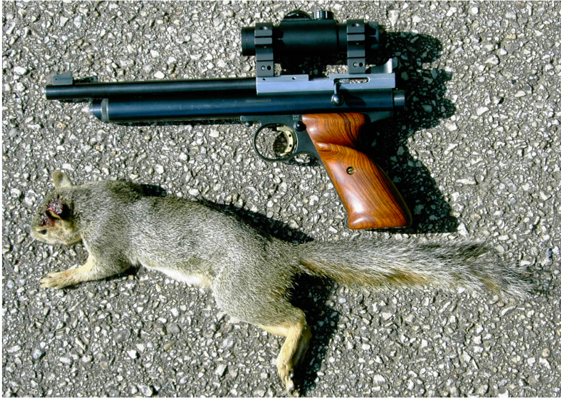
Many current and vintage Co2 pistols can be excellent small-game arms and benefit from simple to elaborate gunsmithing. This .35 caliber custom sports a Crosman trigger and 2250 chamber, bulk filling, Crooked Barn breech, a power adjuster, coco-bolo grips and red-dot scope. It averaged 7/8" groups at 25 yards with 58 grain round balls at 325 FPS/13.6 FP.
