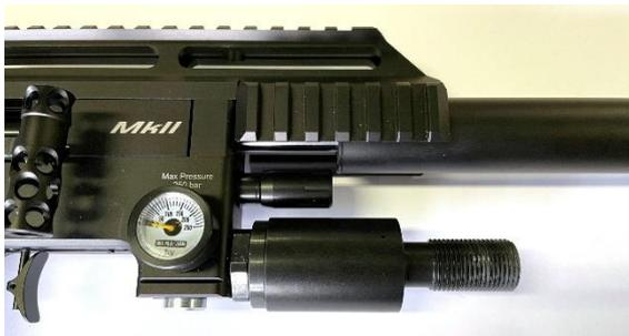
Now place the collar of the regulator on the regulator body. Make sure the blind hole with small measuring hole faces towards the same size as your factory pressure gauge. Then put the o-ring, what you removed from the bottle valve adapter, on the treaded part of the regulator
