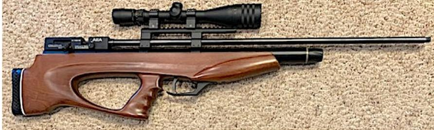
\* I purchased this rifle with the 32" barrel option specifically to **detune** with a weaker hammer-spring, in hopes of achieving a bell-curve power-band. In the tuning process I also installed a lighter trigger spring and moly-lubed the trigger/sear surfaces, reducing the 7 pound, 15 ounce let-off to 2 pounds.
