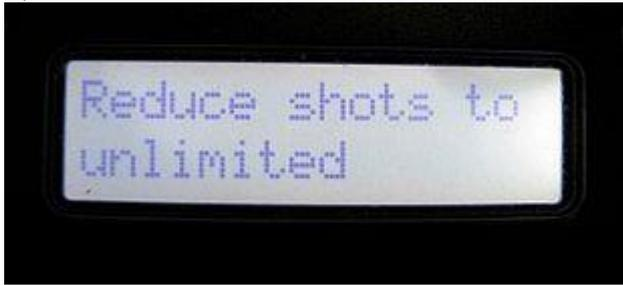
**Hold** the Trigger while switching on. Release when reduce shots menu appears.
