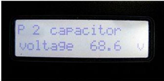
**Hold** the trigger while switching on. Release when capacitor voltage menu appears.
