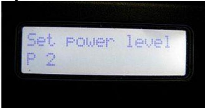
**Hold** the trigger while switching on. Release when power level menu appears.
