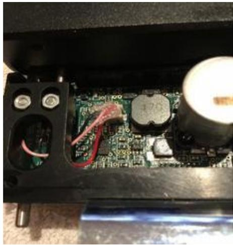
5) Remove the battery cable connector;
