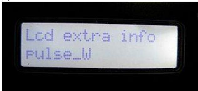
**Hold** the trigger while switching on. Release when LCD extra info menu appears.
