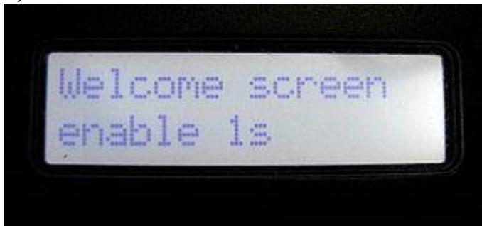
**Hold** the Trigger while switching on .Release when welcome screen Menu appears. **Press** the trigger until desired mode shows. **Hold** the trigger to save the selection.
