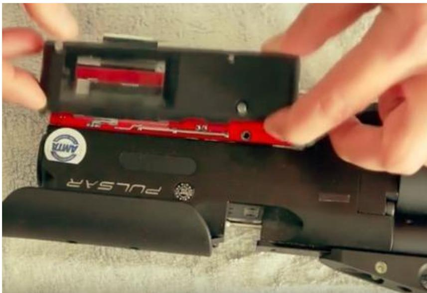
13) Once LCD display side cover secure, gently turn the rifle over and reconnect the far left cable connector;
