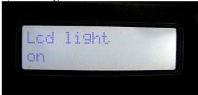
**Hold** the Trigger while switching on. Release when LCD light menu appears.
