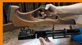
5. When everything's perfectly aligned, fit the BAR bullpup stock.
