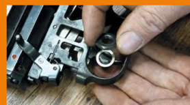
4. Drop the washer over the threaded trigger fixture and secure with the nut.
