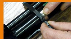
3. Sliding the metal shim into position between the air reservoir and the rear barrel support.
