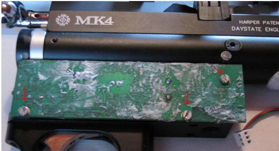
4) Carefully unplug the daughterboard from the mainboard only. Note: The daughterboard will still be connected to the LCD ribbon cable.
