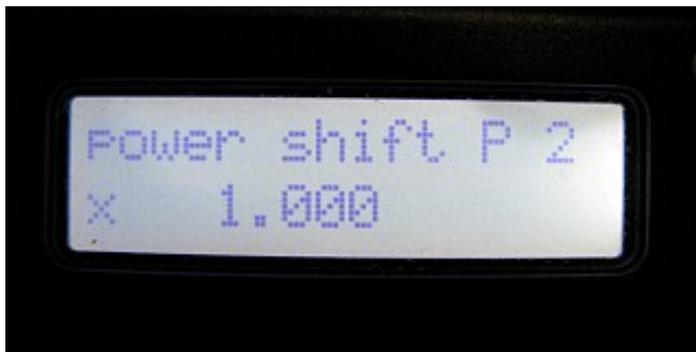
This setting affects the selected power level only. (The power level is selected in menu option #1. The example above shows power level “P 2” being adjusted.)
