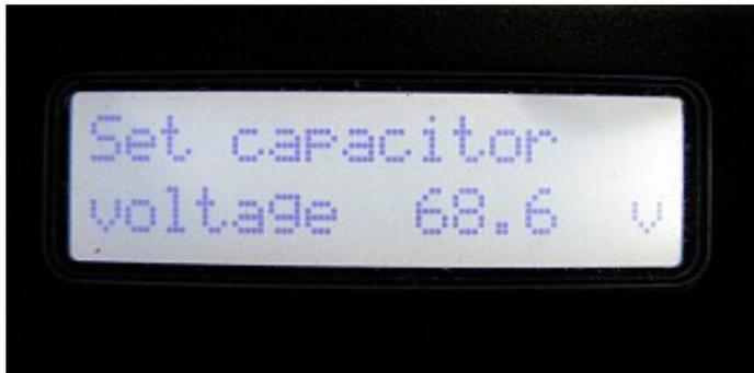
**Press** the trigger until desired voltage shows. The voltage will increment in 0.1v steps. Once the maximum setting is reached, the screen will return to the minimum voltage.
