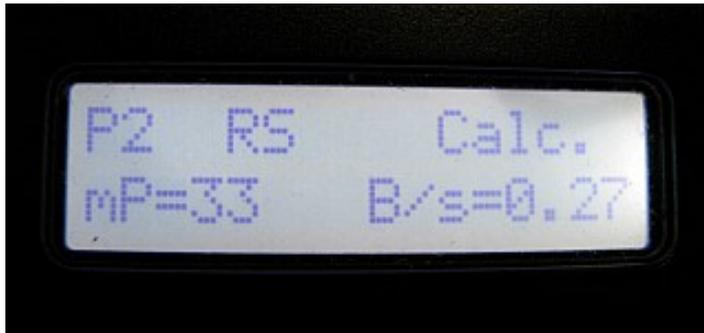
This menu allows for you to make adjustments to the remaining shots calculator for each Power Level.
