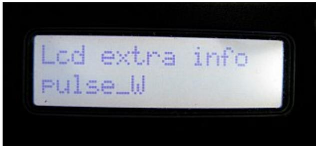
**Press** the trigger until desired mode shows.
