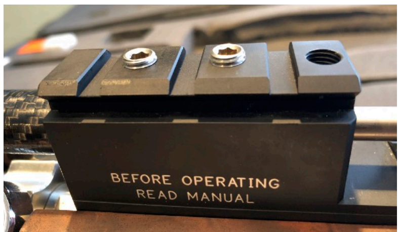
Fig 4: Loosened Barrel Set Screws.
