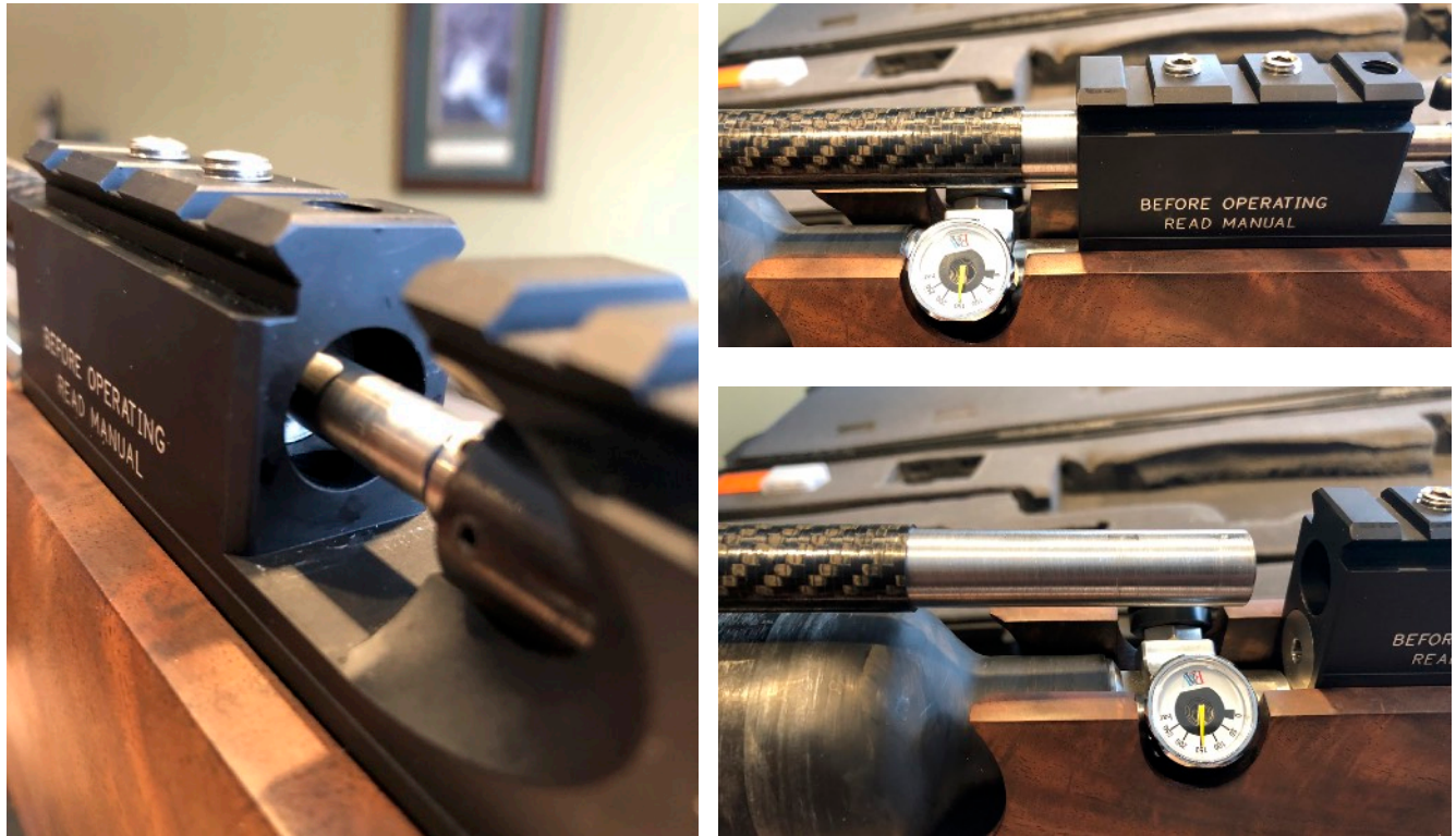
Figs 5-7: Removing Barrel From RAW Action
