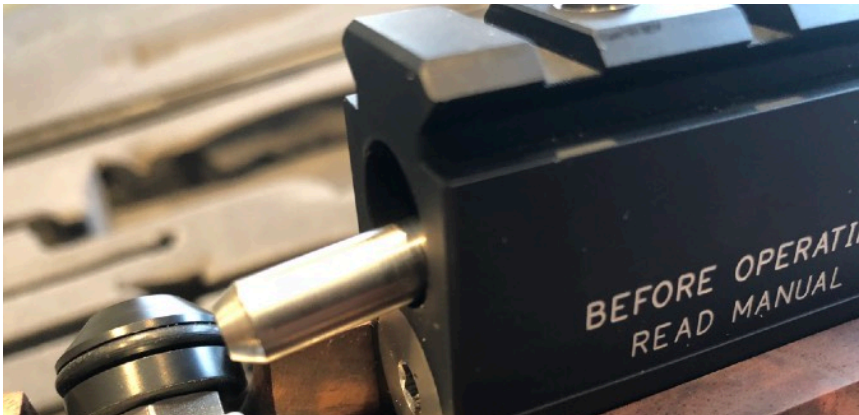
Figs 9: Removal of Probe thru front of Action.
