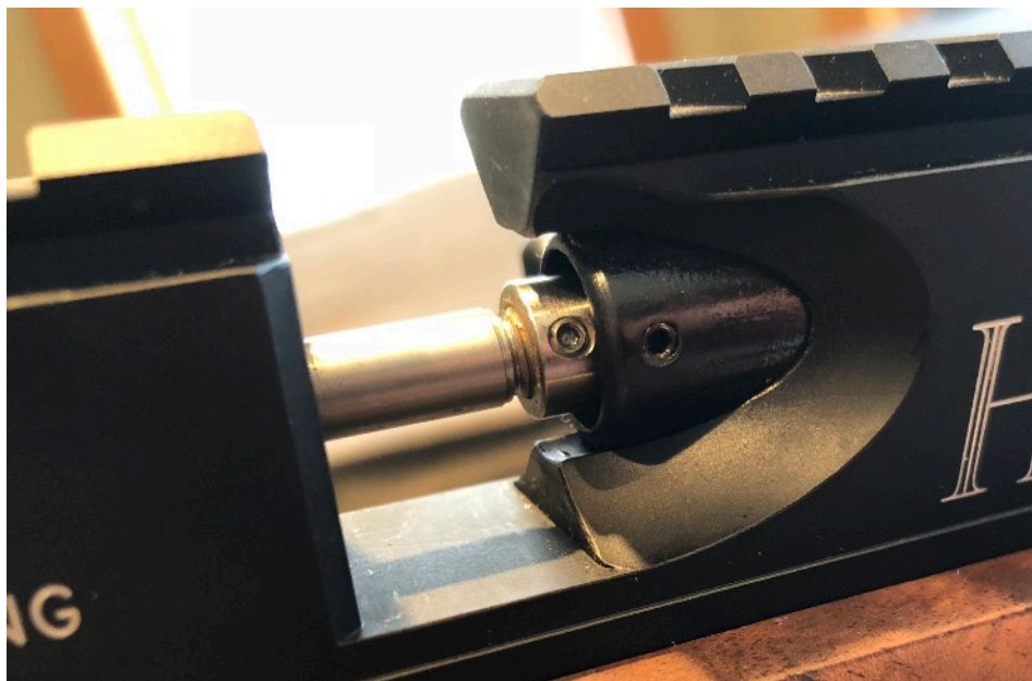
Fig 11: New Probe Installed in Bolt Body.
