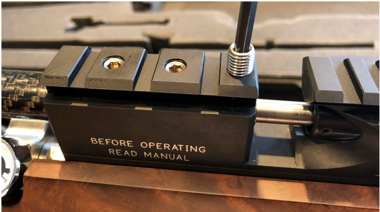
Fig 3: Removal of Rearmost Barrel Set Screw.
